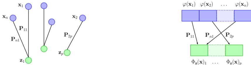
Figure 2: The input point cloud x is transported onto the reference z = (z_1, \dots, z_p) (left), yielding the optimal transport plan P_{\kappa}(x, z) used to aggregate the embedded features and form \Phi_z(x) (right).
